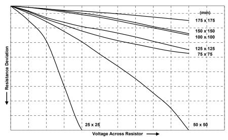
Figure 2a: VCR dependence on resistor geometry
