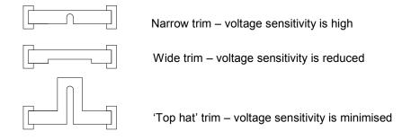
Figure 2d: VCR dependence on trimming geometry
