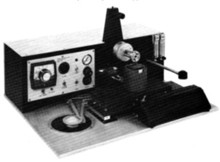
The Model 135 Eutectic Die Attacher is a machine for bonding dice to packages or substrates. The bonding is done on a heat column that heats the package or substrate and a heated pick-up tip, for the dice. To enable the operator to concentrate on placement of the dice, locating motions are mechanized and some operations are performed automatically in sequence.
