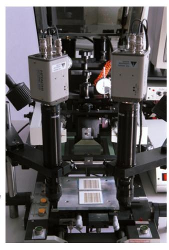
advantages. The printer can accommodate a wide range of substrates from ceramic to epoxy/glass, and materials ranging from cermet and polymer thick film to solder paste, epoxies, and solder mask. The SP-1500 printer has Contact/Off -Contact printing capability, and accepts all standard screen and stencil frames.
