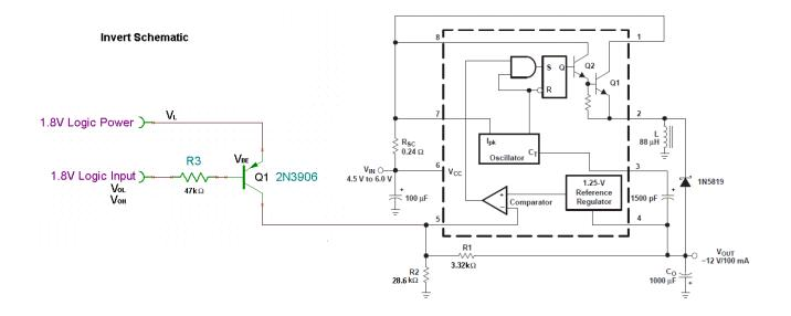
For the inverting regulator, two components (R3&Q1) are needed to disable the MC34063A and shut down the -12V output. When the logic input is high, Q1 is cut off and no collector current will flow. Therefore, Q1 has no effect on the output voltage. When the logic input is low, current will flow through the Q1 base emitter junction. With sufficient base current, Q1 will pull pin 5 (Cii) voltage close to the logic supply voltage.
