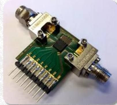
Phase-Shifter 7.5 - 13 GHz RMS Phase Error 1.7° @ 12 GHz Plastic QFN 5x5
