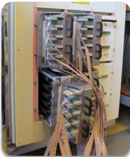
High temperature DC life test
