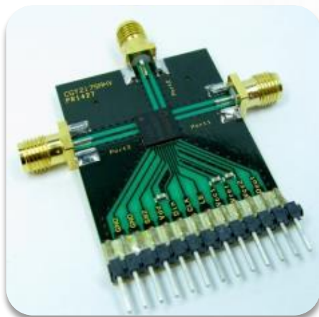
6 bit C-band Corechip Plastic QFN 7x7
